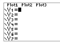
Clear any existing equations by highlighting the row and pressing **CLEAR**. Also make sure that the plots at the top are not highlighted.
