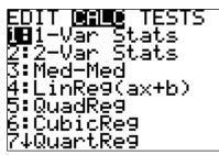
Press **STAT** and highlight the **CALC** column. When you scroll downward, you will see several choices. Number 5 does quadratic regression, finding the best fitting parabola for a set of data. We are going to use number 4.
