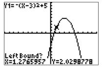
Remove the line from the graph. Now go back to the **CALC** menu ( $2^{nd}$  **TRACE**). Select option 4 to find the maximum. You are prompted. This time you need to give the interval in which the calculator will look for the maximum; i.e., a left bound and a right bound, with the high point in between.
