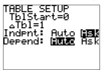
Having the independent variable on 'ask' will allow you to make your own table of inputs and outputs for specific equations.
