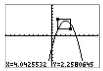
Let's say you want to look at the region near the top of this curve. In the **ZOOM** menu, select option 1. You will see a cursor flashing at the origin. Move it to a position to form a corner of your box and press enter. Now, using the arrow keys, drag out the appropriate box.
