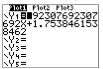
There is an alternative to manually typing this equation. After selecting linear regression and before pressing enter, press **VARS**, select **Y-VARS**, select (1), select (1) again, and then enter. This will tell the calculator to automatically send the regression equation to  $Y_1$ . Note that this gives more decimal places, as shown above. 8) Select 4 and press enter.
