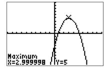
So the maximum occurs at the point (3,5), as we approximated earlier. Note that the value for x is not quite 3. This is due to round-off error. This method is clearly faster than zooming in a bunch of times!
